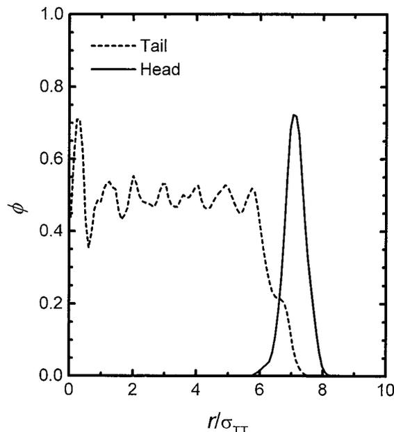
**Figure 2.** Radial variation of the volume fraction ( $\phi$ ) of the tail (dashed line) and head (solid line) groups in a spherical assemblage obtained after equilibration. The lines were averaged over 5000 MC steps after attainment of equilibrium. The axial coordinate is scaled with the tail group diameter. The results were obtained using the potentials described in Section 2 and Table 1.
