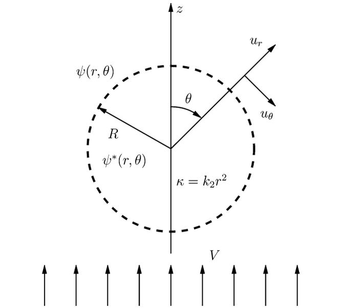
Fig. 1. Coordinate system for axi-symmetric flow relative to an isolated ideal aggregate with quadratically increasing permeability.
