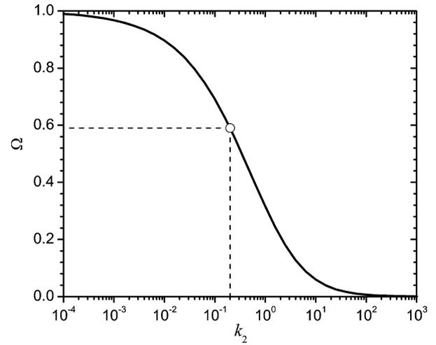
Fig. 4. Variation of the dimensionless hydrodynamic drag force  $\Omega$  with the permeability prefactor  $k_2$ . The hollow circle signifies  $\Omega = 0.59$  with  $k_2 = 0.20$  of the DLCA aggregate (see Section 3.1 for details).
