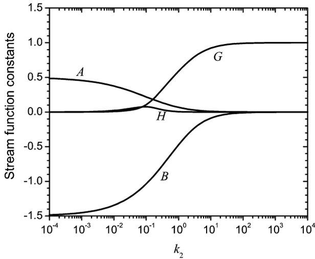
Fig. 3. Variation of the stream function constants  $A$ ,  $B$ ,  $G$ , and  $H$  of Eqs. (23) and (24) with the permeability prefactor  $k_2$ .
