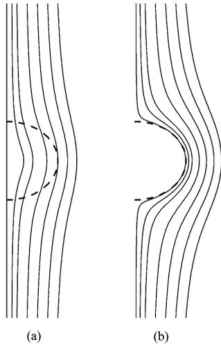
Fig. 5. Streamlines (a) inside and outside the ideal aggregate with  $k_2 = 0.20$ , and (b) outside the solid sphere (i.e., with  $k_2 \rightarrow 0$ ).
