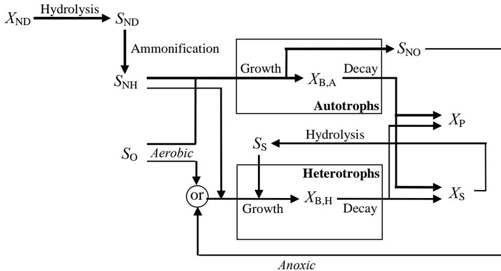
Fig. 2. Diagram of model processes and substrate flow in ASM1.
