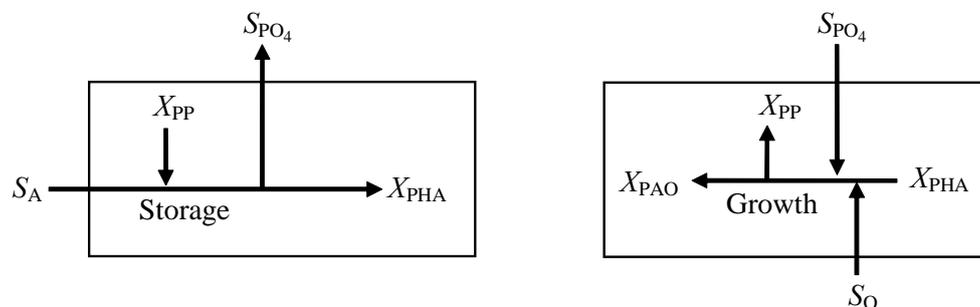
Fig. 3. Storage and growth processes involving PAO in ASM2 (modified from [2]).
