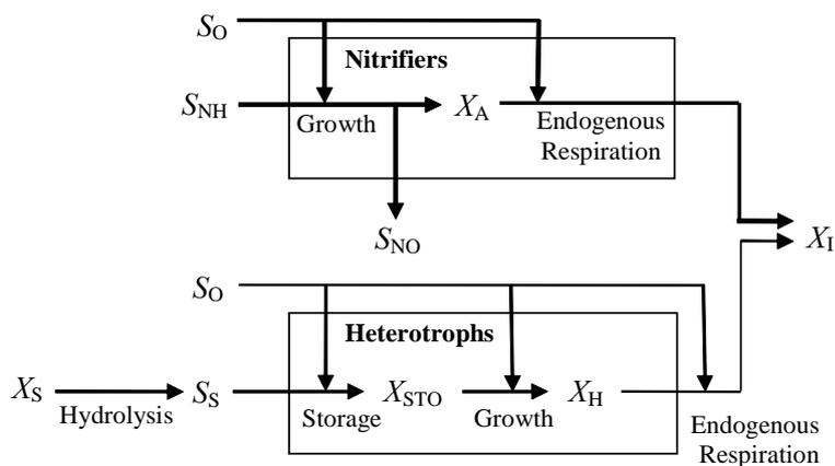
Fig. 4. Diagram of substrate in ASM3 (modified from [8]).
