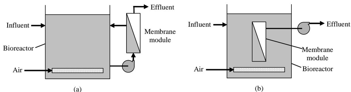
Fig. 1. Schematic diagrams of basic membrane bioreactor configurations [3]: (a) MBR with external membrane module and (b) MBR with immersed membrane module.
