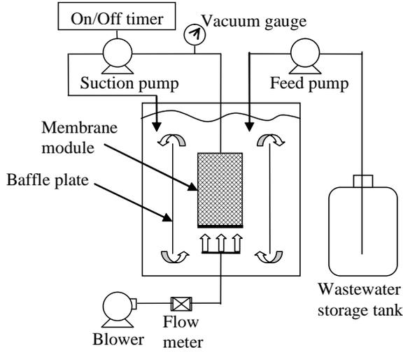
Fig. 6. Diagram of internal-loop-airlift reactor [23].
