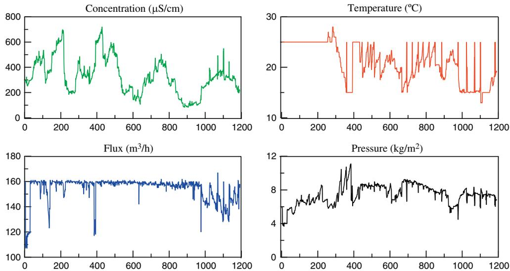
**Fig. 4.** Three-and-half-year membrane filtration operational data for permeate flux, pressure, feed concentrations, and temperature from Woongjin Chemical Co., Ltd. (Seoul, Korea).
