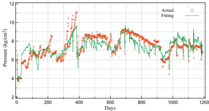
Fig. 7. The comparison of simulated pressure with actual data based on the model described by Eq. (9). The circles denote the actual operational data and the line represents the result from fitting. Parameters used in Eq. 9 are  $\beta_p = -5.304$ ,  $\beta_j = 1.470$ ,  $\beta_c = 9.362 \times 10^{-2}$ ,  $\gamma = 3.206 \times 10^{-2}/^\circ\text{C}$ , and  $\omega = 2.031 \times 10^{-3}/\text{day}$ , which are all significant with  $R^2 = 0.6190$ .
