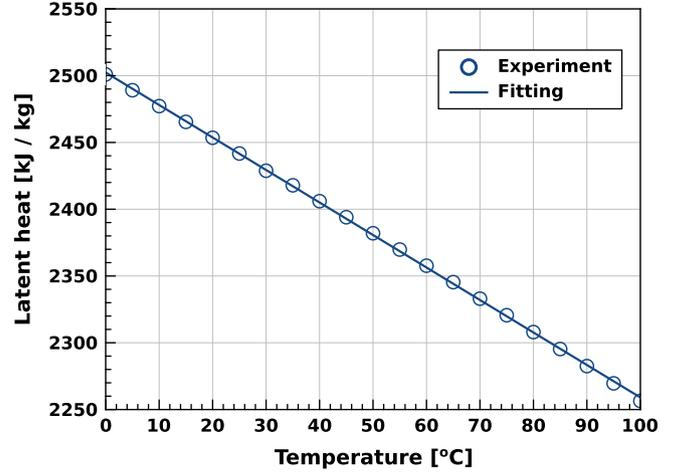
Fig. A1. Latent heat (enthalpy) of liquid water per mass versus temperature, i.e., the heat needed to be adsorbed for water evaporation at a given temperature  $T$ . The solid line is obtained from the linear regression using Eq. (A.4). Data are from Ref. [23].
