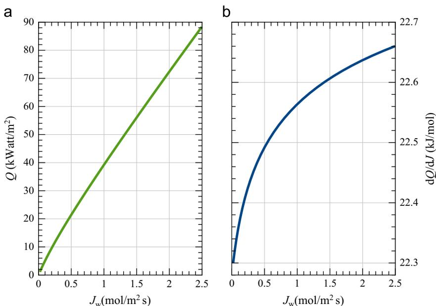
Fig. 6. (a) Heat flux  $Q$  and (b) its derivative with respect to vapor flux  $J_w$ .
