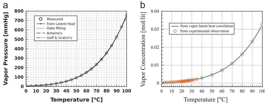
**Fig. A2.** Variation of (a) water vapor pressure and (b) concentration versus temperature. The vapor pressure representation (of Eq. (A.8)) derived from the water latent heat profile has a good agreement with the measured data obtained from Ref. [23]. Fitting Eq. (A.9), Antoine's Eq. (A.10), and Goff-Gratch Eq. (A.11) (of Ref. [24]) also provide equal accuracy.
