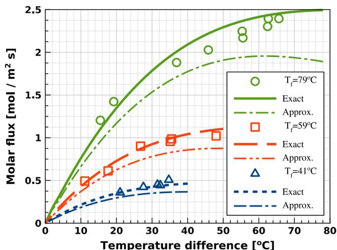
Fig. 4. Comparison of theoretical prediction of water vapor fluxes with experimental observation [7] with respect to the temperature difference at feed temperatures of  $T_f = 79^\circ\text{C}$ ,  $59^\circ\text{C}$ , and  $41^\circ\text{C}$  using 3ME membranes.
