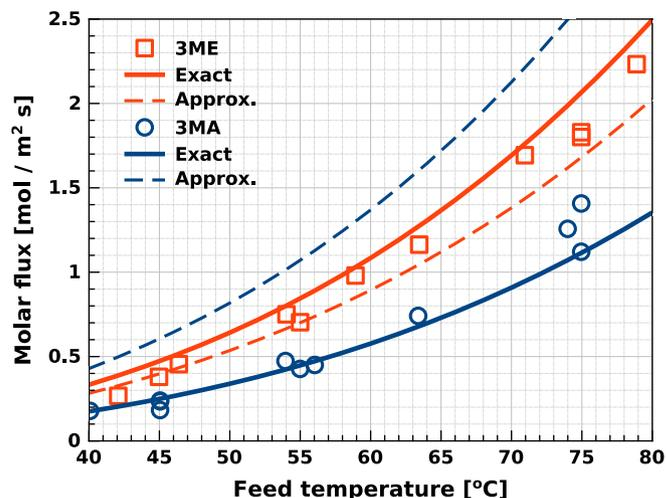
Fig. 3. Comparison of theoretical prediction of water vapor fluxes with experimental observation [7] with respect to the feed temperature at permeate temperature of 25 °C. Symbols and lines indicate experimental and theoretical results using 3MA ( $\epsilon_{max} = 0.66$ ,  $d_p = 0.29 \mu\text{m}$  and  $\delta_m = 91 \mu\text{m}$ ) and 3ME ( $\epsilon_{max} = 0.85$ ,  $d_p = 0.73 \mu\text{m}$  and  $\delta_m = 79 \mu\text{m}$ ) membranes.
