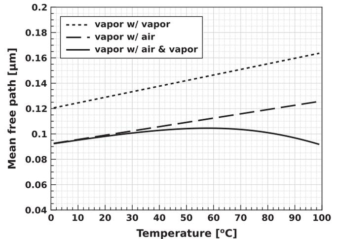
Fig. A3. Estimation of mean free path of water vapor. The dotted and dashed lines indicate that water molecules collide with other water vapor molecules (Eq. (A.14)) or air molecules (Eq. (A.15)) only, respectively; and the solid line represents the effect of water vapor fraction in the gas phase on its mean free path using Eq. (A.19). Decreasing temperature from feed to permeate interfaces is equivalent to increasing axial distance  $z$  from 0 to  $\delta_m$  as indicated in Eq. (6).
