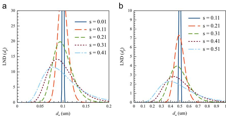
Fig. 7. Pore size distribution (a)  $\langle d_p \rangle = 0.1 \mu\text{m}$  and (b)  $\langle d_p \rangle = 0.5 \mu\text{m}$  with various  $s$ .
